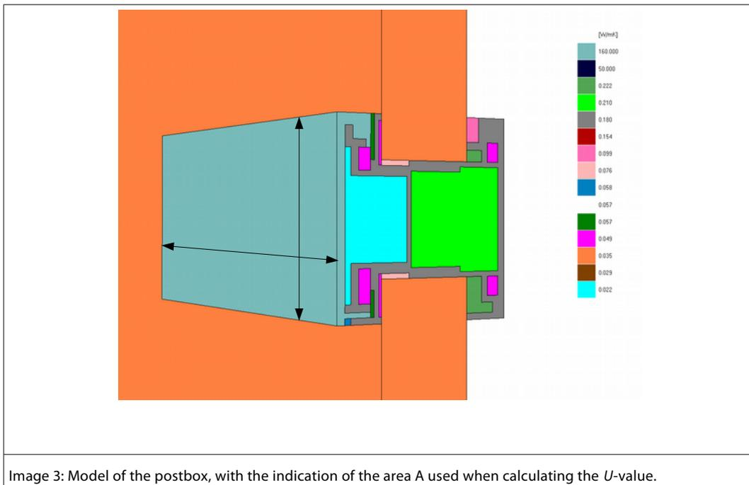
The connection of the postbox to the door leaf, the latter represented by a thermally insulated panel, is shown in image 3. In the model as well as with regard to the calculation of the  $U$ -value of the postbox, the relevant transmission area i.e. calculation boundary is shown by means of the arrows in picture 3.
