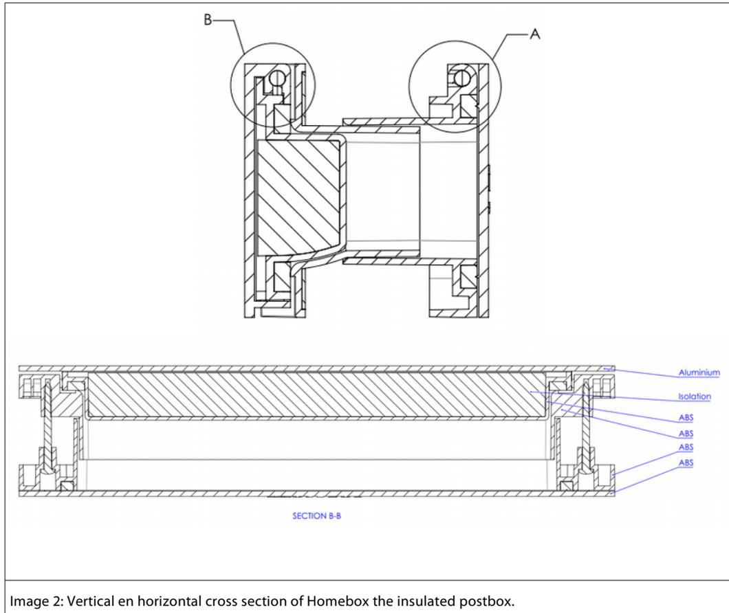
Image 2: Vertical en horizontal cross section of Homebox the insulated postbox.
